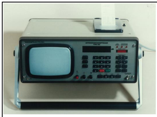
AMA 202 / with automatical level correction and attenuation 1987
